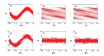
Figure 4: Evolution of the longitudinal phase space in TMC scheme.(a)-After the first modulator; (b)-After the first chicane; (c)-After the second modulator; (d)-After the second chicane; (e)-After the third modulator; (f)-After the third chicane.
