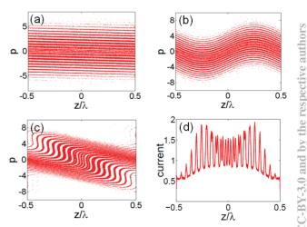
Figure 3: Evolution of the longitudinal phase space in EEHG scheme. (a) after the first strong chciane; (b) after the second modulator; (c) after the second weak chicane; (d) density distribution after the second chicane.
