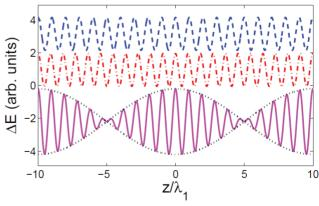
Figure 6: Energy modulation with a laser at  $\lambda_1$  (blue line) and at  $0.9\lambda_1$  (red line); a combination of the two energy modulations (magenta line); the black dotted line illustrates the envelope of the slow modulation at the difference frequency of the two lasers.
