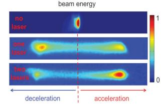
Figure 7: Benefits of cascading in an optical IFEL: a relativistic electron beam with small energy spread (top) can be accelerated with a co-propagating laser (middle), or with two lasers in sequence (bottom).
