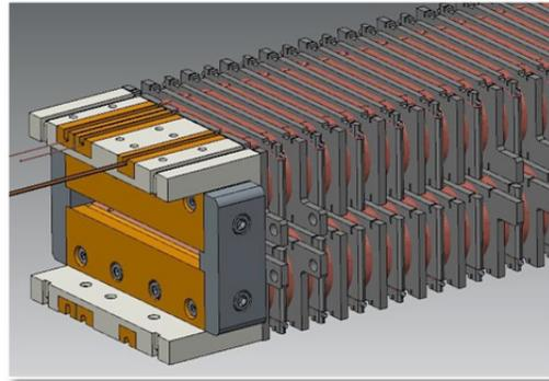
Figure 4: Nb<sub>3</sub>Sn prototype undulator magnet design.
