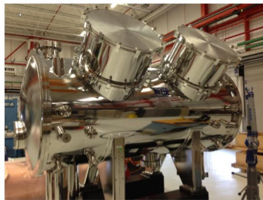
Figure 6: ANL cryostat for testing each of the SCU magnets.
