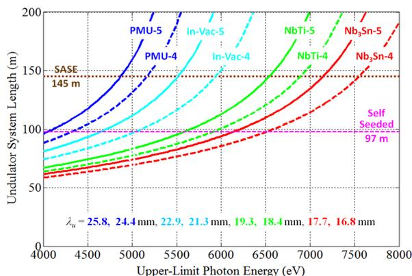
Figure 1: Undulator system length (with breaks) versus upper-limit SASE photon energy saturating in 80% of that undulator length at 4 GeV. Existing 145-m und. hall length is indicated.
