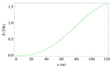
Figure 2: Peak power (1.6 TW) at 4 keV using same “Nb<sub>3</sub>Sn-4” undulator of Figure 1, but now self-seeded, tapered, and driven by the Cu-linac at 6.6 GeV with 4 kA (see Table 1). Segment lengths are 2 m long, which is optimal for this 1-m gain length.
