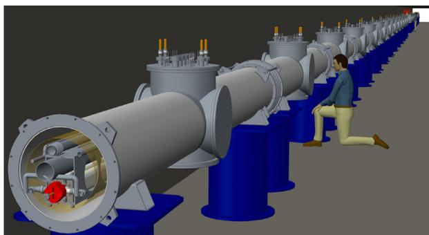
Figure 7: Conceptual SCU system layout for LCLS-II HXU.
