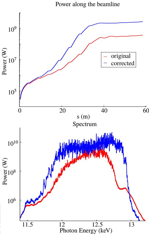
Figure 2: Genesis simulations for the SwissFEL large bandwidth mode at  $\lambda_{\text{photons}} = 1 \text{ \AA}$ . The top picture shows the FEL power for the corrected and the uncorrected case. The resulting increase in FEL power is about one order of magnitude. Uncorrected configuration exhibits narrower spectra, counteracting the goal of the large bandwidth mode.
