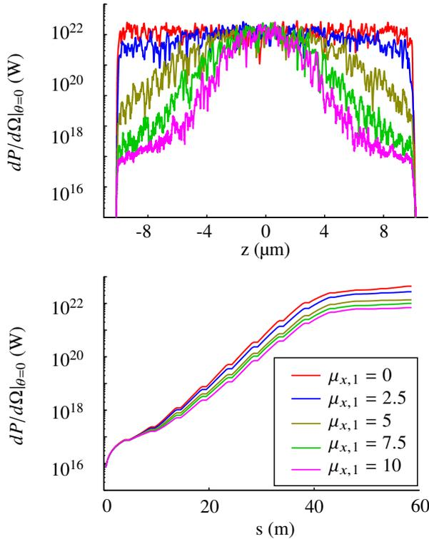
Figure 1: Scan of  $\mu_{x,1}$ . The bottom graph shows the radiation growth along the SwissFEL undulator line whereas the top one represents a snapshot along the FEL pulse at the end of the undulator line.
