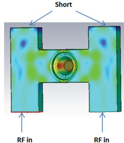
Figure 13: Electrical fields in the H-feed coupler.
