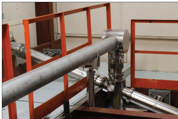
Figure 4: Optical beamlines for the first and the second stage FELs. Radiation of both FELs is delivered to the same user stations. Switching between FELs is done by retractable mirror.
