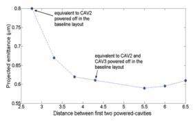
Figure 6: Emittance vs. distance between first two powered-cavities for 300 pC.
