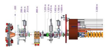
Figure 3: Schematic of new baseline layout from the cathode to CM. Major components are 186 MHz RF gun, two pairs of solenoid/BPM, 1.3 GHz NC RF buncher, ion pump, laser injection box, current diagnostic ICT, YAG screen, two valves, and standard 8-cavity CM.
