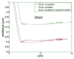
Figure 5: Emittance evolution with perfect RF field (blue), with RF couplers field (green) and correction using a weak skew quadrupole (red) for 300 pC.
