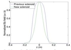
Figure 2: Magnetic field  $B_z$  along z for new and CDR solenoids.
