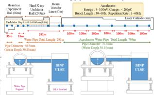
Figure 6: The length and diameter of a water pipe.
