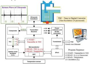
Figure 9: Block diagram of the ULSE Electronics.
