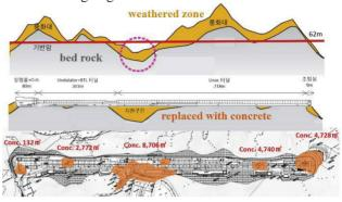
Figure 11: Conditions of creating the PAL-XFEL foundation.
