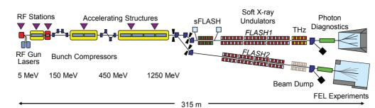
Figure 2: Schematic layout of FLASH user facility. The electron bunch is laser-manipulated in a combination of modulator and chicane installed in the *sFLASH* experiment.
