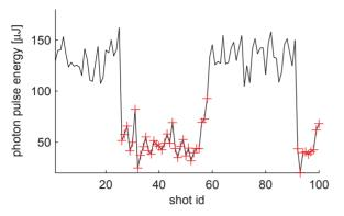
Figure 4: Suppression of FEL lasing for moderate initial laser modulation. The photon pulse energies emitted by the electron bunches have been measured with the GMD detector. Samples obtained with the modulating laser switched on are marked with *red crosses*.
