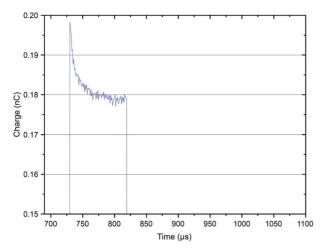
Figure 4: Measured charge along the electron bunch train for a flat laser pulse train as shown in Fig. 5. The bunch to bunch distance is 1 us.
