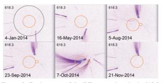
Figure 3: Darkcurrent of the RF-gun with cathode 618.3 and 619.3 measured with a Ce:YAG powder screen during operation in 2014. The red circle indicates the position of the  $Cs_2$ Te film, the black circle the rim of the cathode. The streaks are due to the solenoid field. Pictures were taken under normal operating conditions of the gun (see text).
