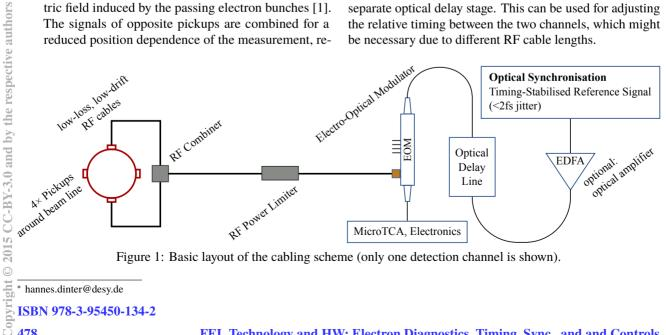
Figure 1: Basic layout of the cabling scheme (only one detection channel is shown).
