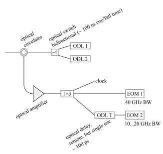
Figure 2: Optical signal processing chain.
