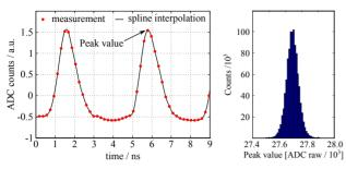
(a) Laser pulse train sampled by scanning (b) Distribution of dethe ADC clock delay. (1000 pulses).
