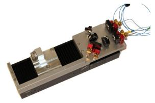
Figure 3: Optical delay stage.
