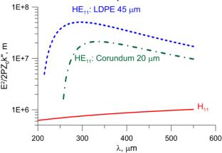
Figure 2: Efficiency of a circular waveguide: all-metal – solid, LDPE coated – dotted, corundum coated – dash-dot.
