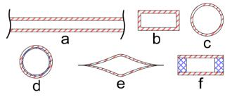
Figure 1: Types of waveguides: a - parallel-plate, b - rectangular, c - circular, d - with dielectric coating, e - special shape, f - rectangular with dielectric walls.
