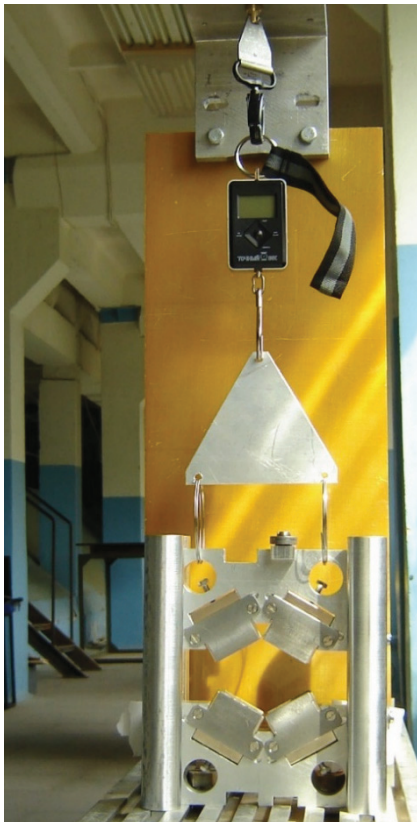
Figure 7: Measurement of the vertical attraction force.
