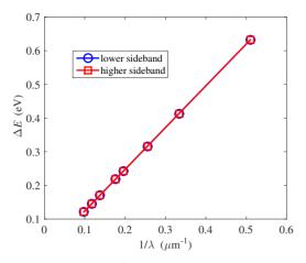
Figure 3: The energy offset of the sideband peaks to the seed versus the inverse of the modulation wavelength.
