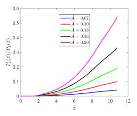
Figure 4: The ratio of the lower sideband to the seed along the undulator for different modulation amplitude.
