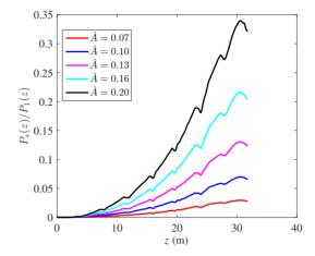
Figure 5: The ratio of the lower sideband to the seed along the undulator for different modulation amplitude in Genesis simulations.
