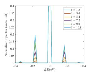
Figure 2: The spectra along the undulator length to illustrate the growth of the sideband power. The spectra are normalized by the power of the seed. The modulation wavelength is 8  $\mu$ m and amplitude is  $\hat{A} = 0.13$ .
