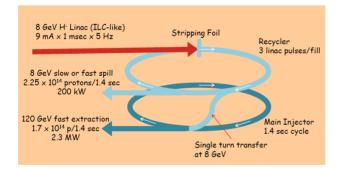
Figure 4: Project X schematic conception for an ILCidentical linac (9 mA x 1 msec x 5 Hz) injecting up to 3 pulses in the Recycler Ring.
