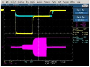
Figure 14a: 13 dB Amplitude Control with Vector Modulator for a 6 kW, 3.5 msec RF Pulse. The purple trace is cavity RF amplitude; the blue and yellow are the vector modulator coils bias currents
