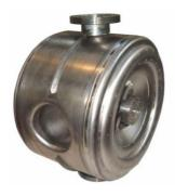
Figure 9: First 325 MHz SSR1 prototype
