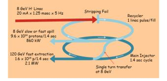
Figure 5: Project X schematic conception for a highpower linac (20 mA x 1.25 msec x 5 Hz) injecting 1 pulse in the Recycler Ring.
