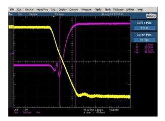
Figure 14b: 120 Degree Phase Control with Vector Modulator for a 300A current change in Vector Modulator coils bias current. The purple trace is the cavity RF phase signal (changing by  $120^{\circ}$  between the 2 vertical purple lines), the yellow trace is the bias currents.
