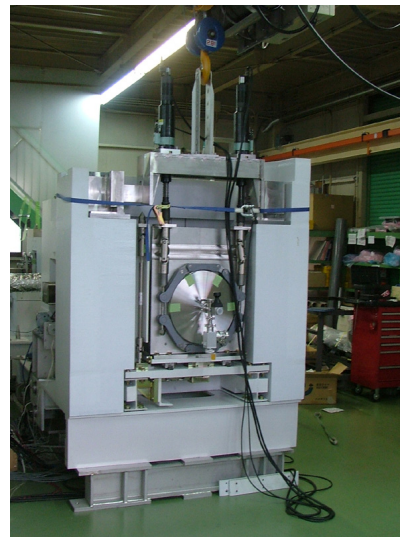
Figure 7: Schematic of the remote clamp system. By using the remote clamp system, the collimator vacuum chamber can be removed only by turning the screws far from the collimator. The quick-coupling clamp can be opened by turning two screws which are connected with the clamp, and the other screw separates the flange of collimator chamber and the flange of other accelerator component.
