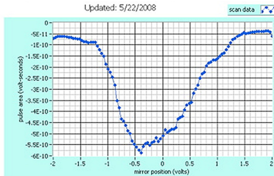
Figure 11: Initial transverse beam profile measurements at BNL of 750 keV H - .
