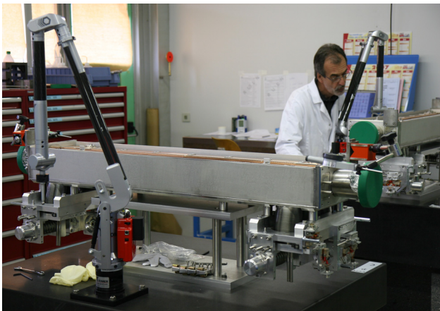
Figure 8: Precision alignment and survey of collimators with installed jaws during production.
