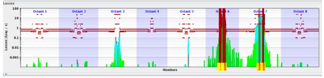
Figure 10. Map of losses through the LHC for asynchronous dump test with about  $3 \times 10^{10}$  p+ in each abort gap. The dumps for Beam 1 and Beam 2 were triggered together. The losses in Octants 3 and 7 are on the collimation insertions, and in Octant 5 on the TCTH which protects the low- $\beta$  triplets. A dump of the full intensity 25 ns beam will give losses about 500 time higher.
