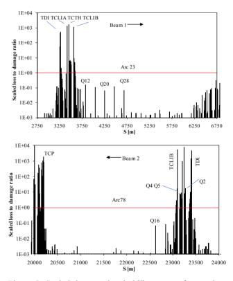
Figure 9. Scaled damage threshold/loss maps for grazing incidence impact on TDIs, for Beam 1 (upper) and Beam 2 (lower).
