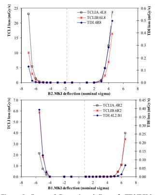
Figure 8. Scans of Beam 1 and Beam 2 TDI/TCLI opening with simulated MKI deflection variation, in sigma. The nominal system opening is  $\pm 6.8$  sigma.
