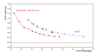
Figure 7. Scale effect between Beam 1 TCP and TDI settings, which could be explained by a TDI gap some 2.4 mm smaller than expected, and the improvement observed when the 900 µrad tilt on the lower TDI jaw was corrected.
