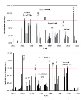
Figure 5. Losses in the injection regions are all on the protection devices and collimators, except for the MKIs, which are a factor 3 above the assumed damage limit.
