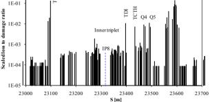
Figure 6. Absolute losses in injection regions for Beam 1 and Beam 2. Losses on the MKIs are lower than those on the adjacent Q4 and Q5.
