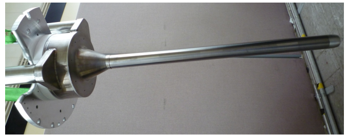
Figure 8: Completed target ready for integration with horn.
