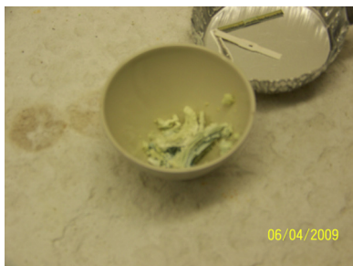
Figure 9: Oxidation of irradiated Ta at 1100°C.
