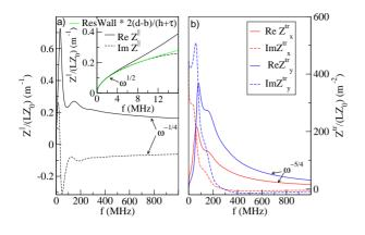
Figure 2: Impedances in the Booster F-magnet. a) Longitudinal impedance. Notice (inset) that at low frequencies the impedance has a  $\omega^{1/2}$  behavior characteristic of resistive wall pipes, but is  $2\frac{d-b}{h+\tau} \approx 385$  larger than the corresponding impedance of an iron pipe. b) Transverse horizontal and vertical impedances.
