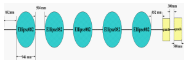
Figure 2: Schematic layout of one cell of the Elliptical082 section.
