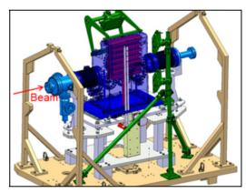
Figure 7: General assembly of the sample holder.
