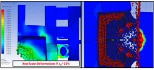
Figures 5-6: Case 7. Plastic strain in Cu and Cu-Ni (left) and damage extension on the two jaws (right).
