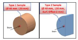
Figures 8-9: Type 1(left) and type 2 (right) material sample shapes.
