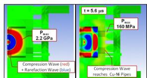
Figures 3-4: Case 4. Propagation of the shock wave in the jaw assembly.
