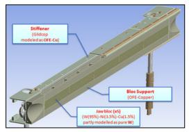
Figure 2: Jaw assembly of a TCT Collimator.
