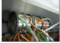
Figure 13: Strain gauges mounted on Inermet® specimens.
