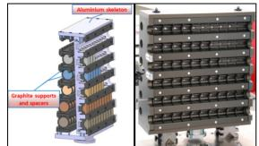
Figures 10-11: Specimen housing of the material sample holder.
