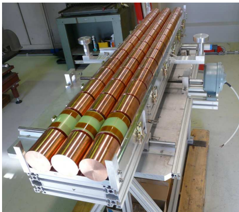
Figure 1: Target with 3 assemblies, each with 15 copper cylinders. The aluminium enclosure and caps are not shown.
