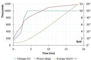
Figure 9: RF acceleration program for the 12 GeV VFFAG.
