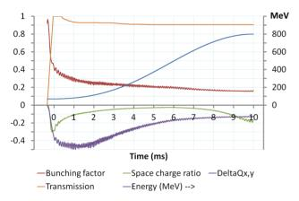
Figure 8: Bunching factor, transmission and intensitydependent effects in the ISIS first harmonic simulation.
