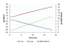
Figure 12: Increase of bunch energy spread in the 12 GeV VFFAG simulation to  $\pm 41.1 \text{ MeV}$ .
