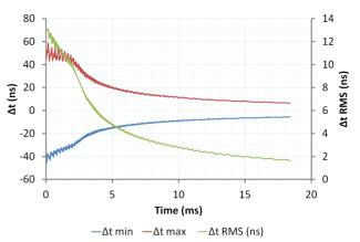
Figure 11: Bunch duration in the 12 GeV VFFAG simulation, reducing to a final value of  $\Delta t_{\rm rms} = 1.64$  ns.
