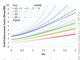
Figure 2: Field enhancements as a function of  $\tau$ , fringe length (f) and distance from mid-plane (x) from 0 to 4 cm, in the 3 or 5 GeV magnet design with  $k = 2.05 \text{ m}^{-1}$ .
