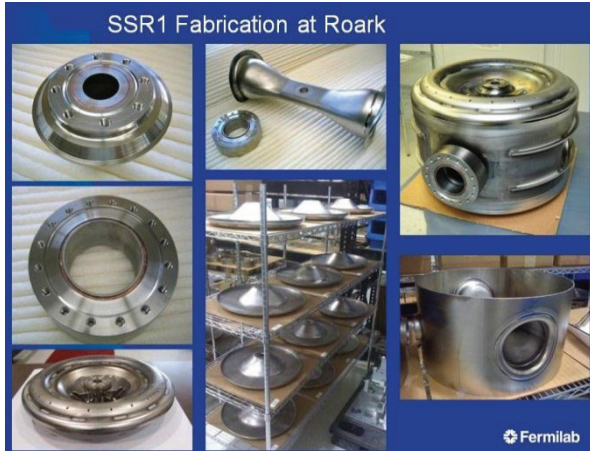
Figure 3: SSR1 cavities in fabrication at Roark.
