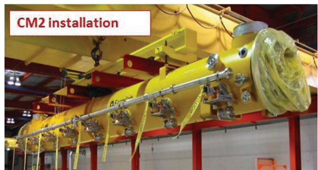
Figure 10: CM2 Installation for testing.
