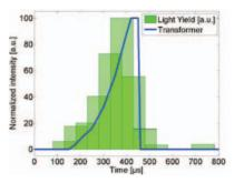
Figure 3: Time response of OTR (green) and transformer signal (blue) of an  $U^{-73+}$  ion beam with 300 µs pulse duration. Every bar shows the OTR signal strength in a shifted 100 µs time window.
