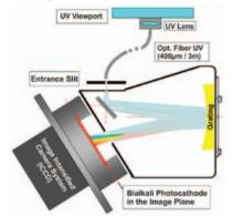
Figure 7: Scheme of the spectroscopic setup.
