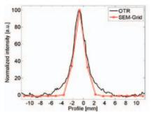
Figure 6: Comparison of the beam profile for two methods: OTR (black) and SEM-Grid (red).
