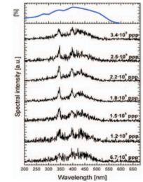
Figure 8: OTR spectra obtained for different  $U^{-73+}$  ion intensities, not normalized or corrected. The spectral efficiency of the Bialkali photocathode is shown in the upper graph (blue line). The spectra were recorded during ~ 500 beam pulses.
