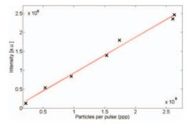
Figure 4: The OTR signal strength as a function of the particle number for the  $U^{-73+}$  beam.
