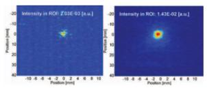
Figure 5: False colour OTR images during irradiation with 6.7·10<sup>8</sup> Uranium ions, without stripping foil (left,  $U^{28+}$ ) and with 570 µg/cm<sup>2</sup> carbon stripping foil (right,  $U^{-73+}$ ). Beam energy is 11.4 MeV/u and pulse length 300 µs.
