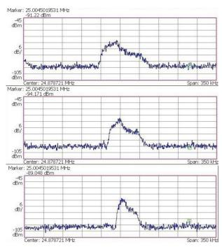
Figure 5: Longitudinal Schottky spectra measured using standard SIS18 Schottky system for different buncher settings: bunching (top), buncher off (middle) and debunching (bottom).
