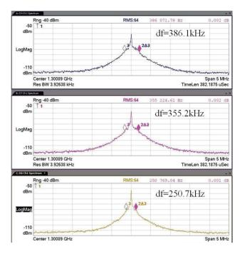
Figure 6: Spectra for Unilac beam measured using new method for different buncher settings. The order is as in Fig. 5.
