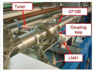
Figure 2: Cavity installed in the transfer beam line between Unilac and SIS18 synchrotron.
