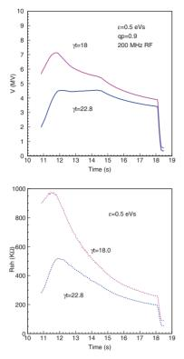
Figure 6: Voltage programs (top) and narrow-band impedance thresholds (bottom) through the cycle for Q26 (blue curve) and Q20 (magenta curve) optics in a single RF system for longitudinal emittance  $\varepsilon_l = 0.5$  eVs. Acceleration starts at 10.86 s.
