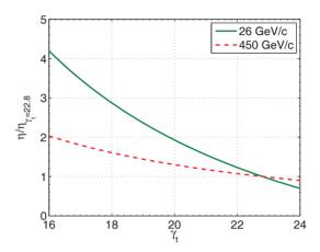
Figure 1: Slip factor  $\eta$  relative to the value of the nominal SPS optics (nominal  $\gamma_t = 22.8$ ) as a function of  $\gamma_t$ . At injection  $\gamma = 27.7$  and at extraction  $\gamma = 480$ .
