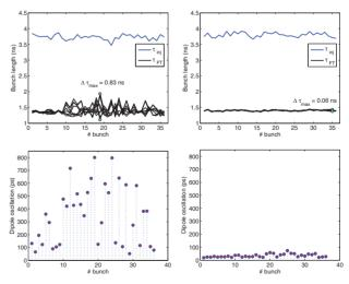
Figure 8: Bunch length (top) and bunch position (bottom) oscillations at flat top for the bunches of a single batch 50 ns LHC beam, for Q26 (left) and for Q20 (right).
