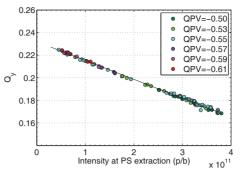
Figure 2: Vertical tune as function of intensity at PS extraction for different settings of the vertical chromaticity knob.
