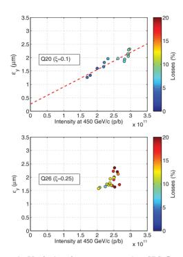
Figure 4: Vertical emittance measured at SPS flat top as function of the intensity for the Q20 optics (top) and the nominal SPS optics Q26 (bottom).
