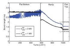
Figure 7: Bunch length evolution along the cycle for single bunches ( $N_b \approx 1.1 \times 10^{11} \text{ p/b}$ ) in Q26 with single RF system for two different capture voltages. The voltage programs after the flat bottom are the same in both cases.
