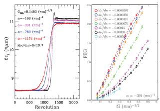
Figure 10: Left: Emittance growth when passing through a third-order resonance at tune-ramp rate  $|d\nu/dn|=6\times 10^{-5}$  and resonance strength  $G=0.1483\,(\pi\mathrm{m})^{-1/2}$  for various detuning parameters. Right: FEG vs resonance strength G for a wide range of tune-ramp rates at initial rms emittance  $\epsilon_i=4.62\,\pi\mu\mathrm{m}$  and detuning  $\alpha=-391\,(\pi\mathrm{m})^{-1}$ .
