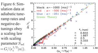
For FFAGs, the adiabatic FEG is too large to be acceptable in practice. The tune-ramp rate usually depends on energy gain per turn, and one often tries to ramp through the resonances as fast as possible. The typical tune-ramp rate is about  $10^{-3} \sim 10^{-5}$  per revolution. Figure 7 shows that the FEG becomes detuning independent when the tune-ramp rate is higher than  $\sim 10^{-5}$ .
