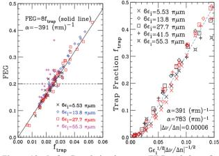
Figure 12: Left: Correlation between FEG and  $f_{\rm trap}$  for  $\alpha < 0$  for beams with different emittances, resonance strengths and tune-ramp rates. Right: Trap-fraction vs scaling parameter S of Eq. (8) for various initial emittances, two detuning parameters, and a fixed tune-ramp rate  $d\nu/dn = -6 \times 10^{-5}$ .
