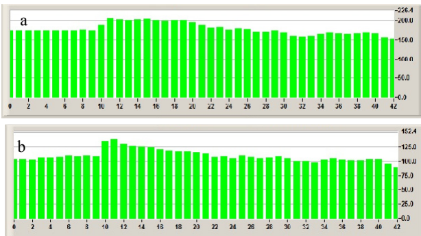
Figure 4: Distribution of auxiliary voltage along the accelerating column. The sections 10-42 correspond to column; the sections 0-9 are high-voltage terminal. The variant (a) is no-load operation of the cascade transformer, the variant (b) is operation at the nominal current in high-voltage sections (2.5 A) and the electron current 0.5 A in the collector.
