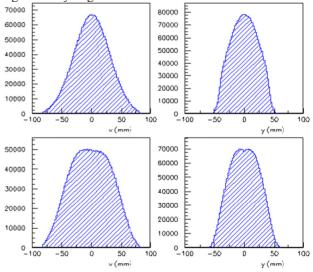
Figure 9: TURTLE Simulation of the proton beam transverse distribution at the SINQ target entrance in normal running conditions (top) and applying a beam rotation system  $\sim 24$  m upstream of the SINQ target (bottom). *x* and *y* coordinates follow the TURTLE convention (*x* is the bending plane) and are therefore reversed.
