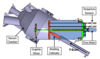
Figure 6: Drawing of the new target M insertion.
