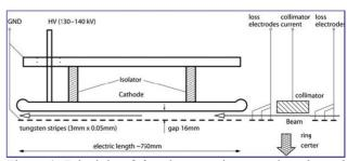
Figure 4: Principle of the electrostatic extraction channel EEC.
