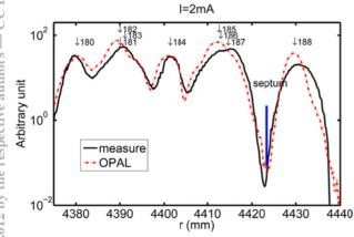
Figure 2: Radial beam profile with turn number at the extraction.
