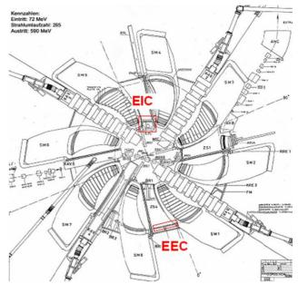
Figure 3: Drawing of the PSI ring cyclotron. The red elements are the electrostatic injection/extraction channels (EIC/EEC).
