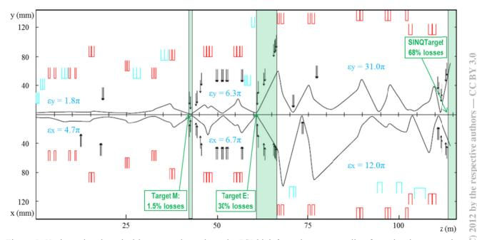
Figure 5: Horizontal and vertical beam envelops along the PSI high intensity transport line from the ring extraction. Beam emittances  $(2\sigma)$  are expressed in unit of mm mrad and refer to the non-dispersive component.
