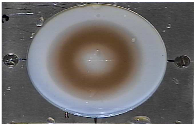
Figure 1: Measured beam at the IPF target by foil irradiation: 300 s exposure time at 2 Hz, 7 \mu A average current.
