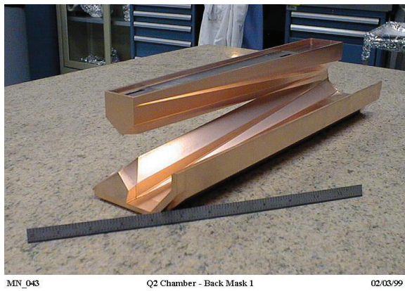
Figure 11:Q2 chamber showing taper, masking and heavy duty water cooling with tapered sided to reduce local synchrotron radiation heat loading and stresses (S. Ecklund, N. Kurita).
