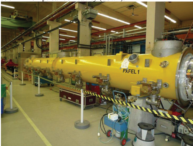
Figure 11: 12 meters long cryomodule for Euro-XFEL .
