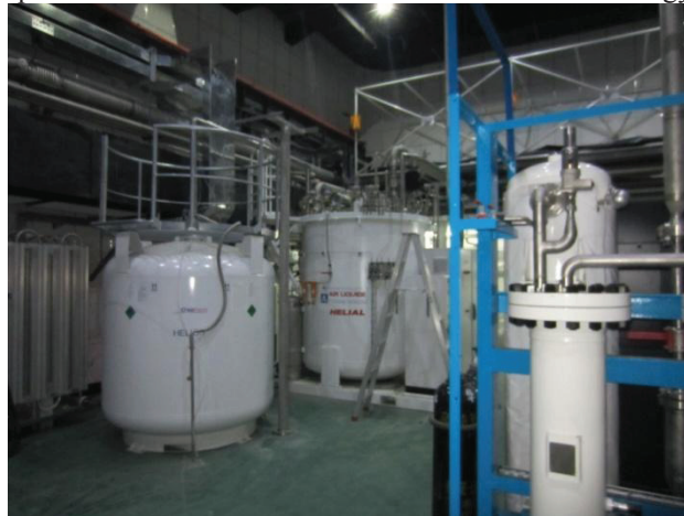
Figure 12: 2K cryogenic LHe system.
