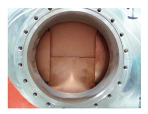
Figure 6: The four Copper plates, making one Slit monitor, installed on their tank. Left and right plates are positioned at beam border; top and bottom plates are making a very thin slit at about tank center.
