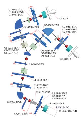
Figure 1: LEBT line layout. Sketch of magnets and beam diagnostics monitors, from the sources to the test bench installed at the end of the LEBT line, during LEBT commissioning, in place of the RFQ. Legend: SLA= Slit monitor, FCA= Faraday Cup monitor, BWS= Wire Scanner, CFC= Chopper Faraday Cup monitor, GCT= AC- Current Transformer, PIA= Wires Harp, IC1= Chopper magnet.
