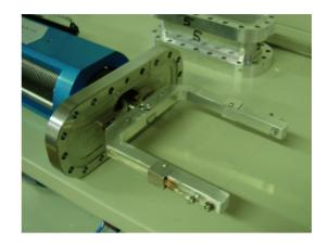
Figure 2: Picture of the Wire Scanner monitor wire, mounted on its fork. Wire fork is screwed to the brushless motor shaft that drives the wire IN /OUT the beam path.
