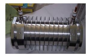
Figure 5: Chopper Faraday cup body, that is the vacuum chamber section just behind the Chopper magnet. Thin metallic tabs are machined on the body itself, in order to enhance heat evacuation by air-convection.
