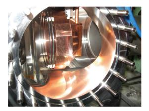
Figure 4: Faraday cup monitor installed on its tank and looked at from a side port (beam should come from the left). One can recognize the Copper cup, from its typical colour. Two stainless steel rings are mounted in front of the cup: the repeller ring (on the left), and the guard ring (on the right).
