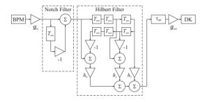
Figure 3: Block diagram of feedback loop with the notch and Hilbert filters.
