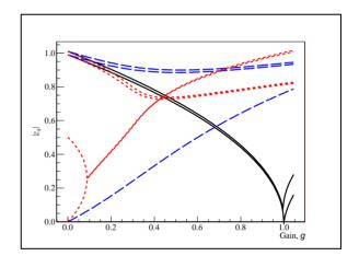
Figure 5: Dependences of damping rates  $|z_k|$  on gain g for the ideal TFS (solid curves), for the TFS with the notch filter (dashed curves) and for the TFS with the notch and allpass filters (dotted curves), parameter a = -0.501; shown is the case of the tune of Q = 6.73 and an assumed instability rise time of  $\tau_{inst} = 100T_{rev}$ .
