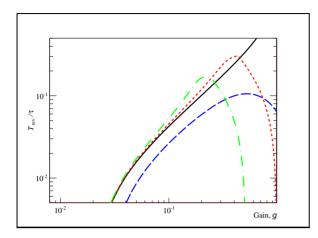
Figure 6: Dependences of overall damping rates  $T_{\rm rev}/\tau$ on gain g for feedbacks: the ideal TFS (solid curve), with the notch filter (dashed curve), with the notch and allpass filters for a = -0.501 (dotted curve), with the notch and Hilbert filters for  $\Delta \varphi = -72.8^{\circ}$  (dash-dotted curve); shown is the case of the tune of Q = 6.73 and an assumed instability rise time of  $\tau_{\rm inst} = 100T_{\rm rev}$ .
