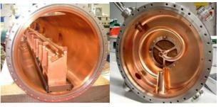
Figure 4: View into the HITRAP 4-rod RFQ and inside the de-buncher integrated into the RFQ tank.
