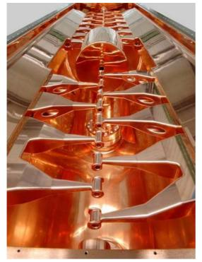
Figure 3: View into the HITRAP IH-structure from the low energy end of the resonator.
