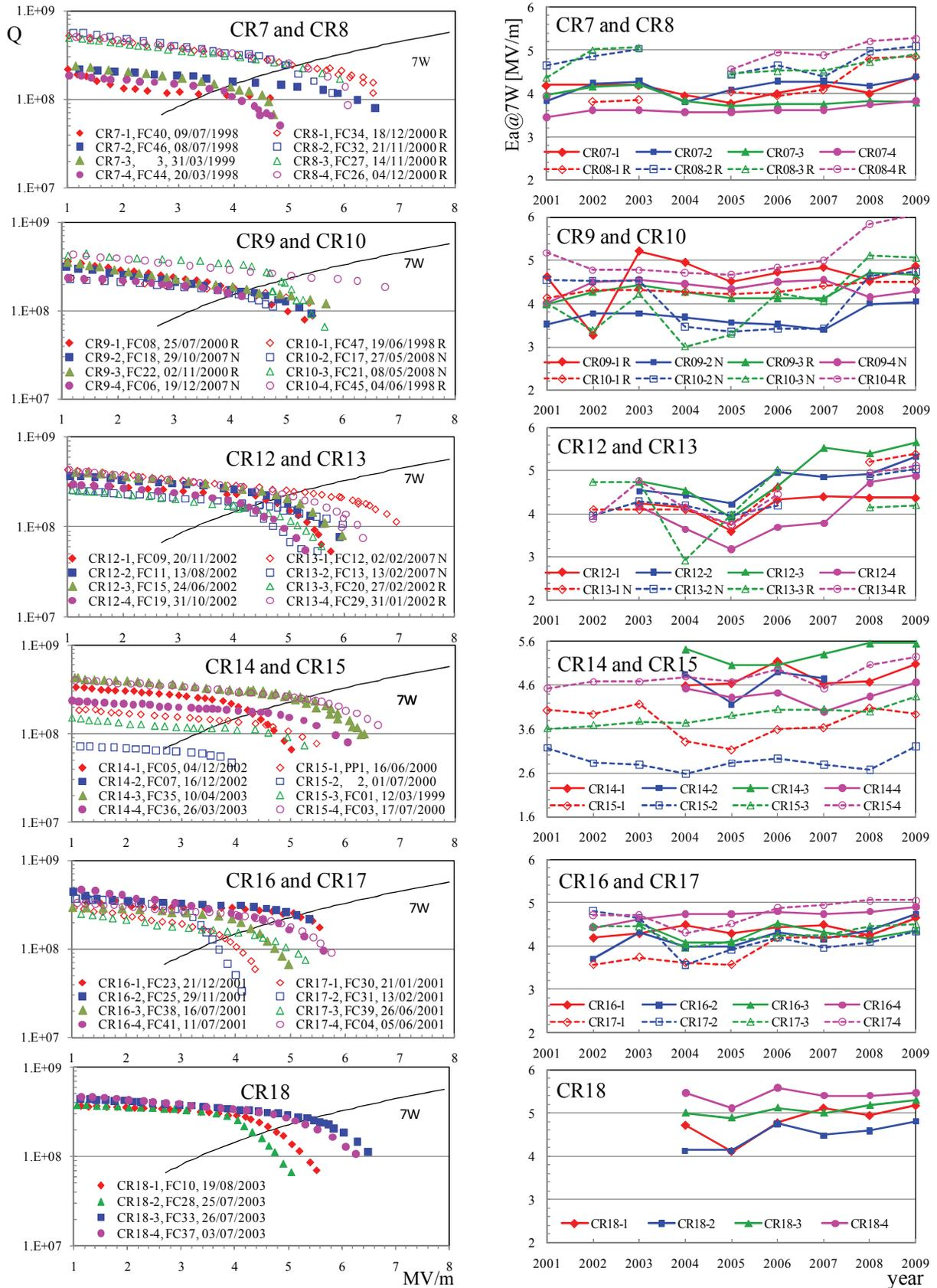
Figure 4: Q curves (left) and performance in the last years (right) of the medium  $\beta$  resonators installed in ALPI cryostats. See text for comments.
