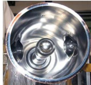
Figure 3: A newly designed medium  $\beta$  cavity.
