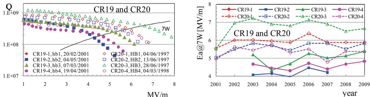
Figure 5: Q curves (left) and performance in the last years (right) of high  $\beta$  resonators installed in ALPI cryostats. See text for comments.
