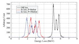
Figure 6: α energy loss in a Silicon detector.
