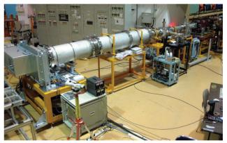
Figure 1: Photograph of the prototype of the raster scanning system.
