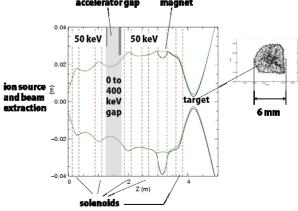
Figure 4: Simulations of the entire DIANA low energy beam transport line using the particle-in-cell code WARP. See text for description.
