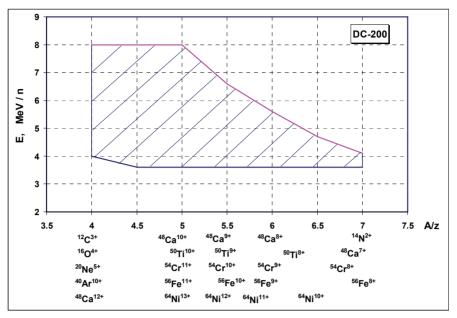
Figure 10: Cyclotron DC200 working diagram.
