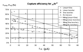
Figure 8: The efficiency of capture versus injecting beam current and bunchers.
