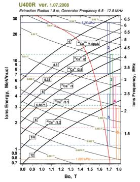
Figure 3: Operating chart of the U400R cyclotron.
