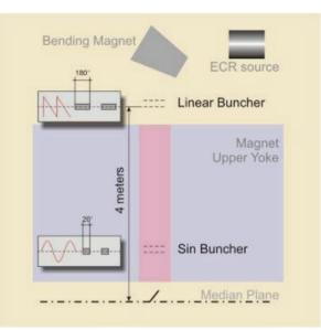
Figure 2: Scheme of the beam bunching system.
