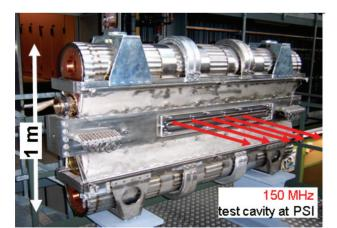
Figure 4: 150 MHZ test cavity (single gap). A 92 MHz cavity is approx 1.5 times higher.
