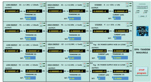
Figure 4: The computer control system for all the electrostatic and magnetic deflectors on the accelerator.
