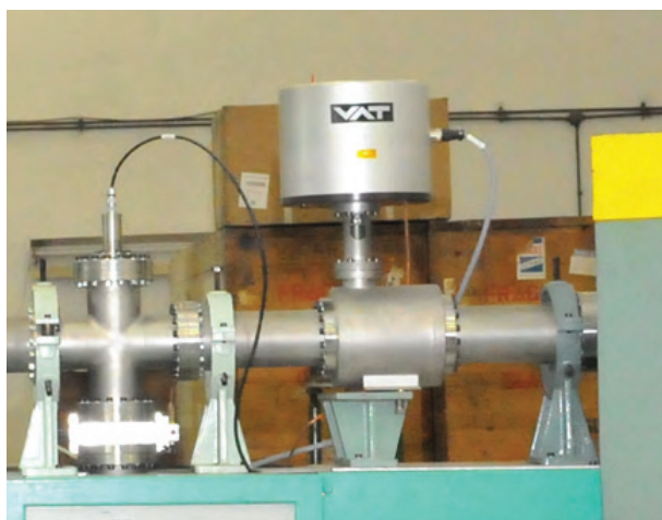
Figure 6: Fast closing valve designed to protect the vacuum pumps and the stripping carbon foils of the accelerator from accidental input of air
