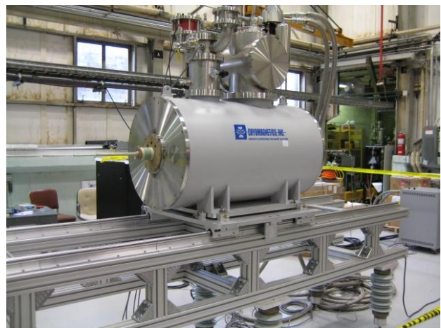
Figure 4: Photograph of 6 T solenoid installed at HV platform.
