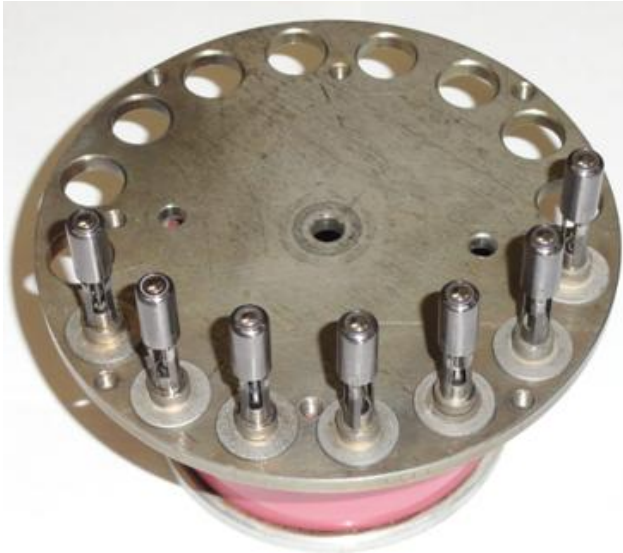
Figure 7: Photograph of 4 mm IrCe thermionic cathode units mounted for heating tests.
