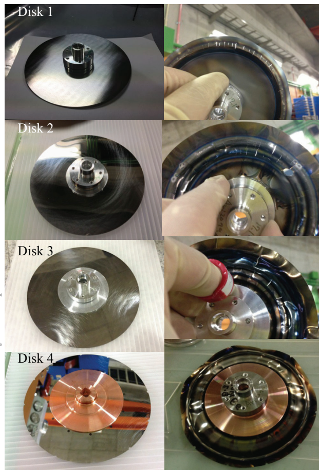
Figure 1: The four Be-disks : before usage (left) and after usage (right).
