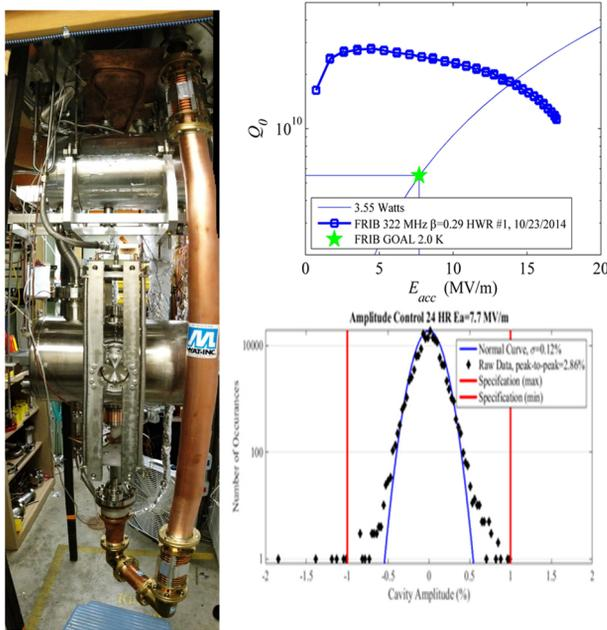
Figure 4: Preparation for 24-hour integrated test of  $\beta_0=0.29$  cavity (left);  $Q_0$  vs.  $E_{acc}$  performance measured at 2 K (top right); and measured RF amplitude control performance at 2 K (bottom right).
