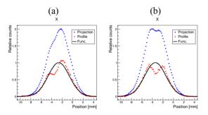
Figure 5: The beam profile before the tuning (a) and after the tuning (b). The red points show normalised line profile. The blue points show normalized projected image. The black line shows the 2D Gaussian distribution.
