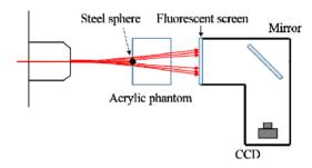
Figure 3: Configuration of the verification system. Light emissions are detected by CCD camera via 45 degree rotated mirror.
