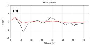
Figure 2: Simulation results of beamline tuning of vertical course for Room2. Horizontal (a) and vertical (b) beam's trajectories are shown. The beam's trajectories before the beamline tuning (Black) and after the beamline tuning (Red) are shown.
