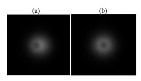
Figure 4: Beam spot images before the beamline tuning (a) and after the beamline tuning (b).
