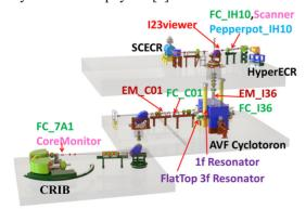
Figure 1: The schematic view of Hyper ECRIS, AVF cyclotron and CRIB with beam transport line.
