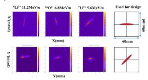
Figure 7: Columns from 1st to 3rd are the measured emittances. 4th column is the emittance used for design. Upper and lower rows indicate respectively a horizontal emittance and a vertical emittance.
